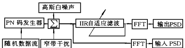
图4 计算机仿真框图 Fig. 4 Block diagram for computer simulation
