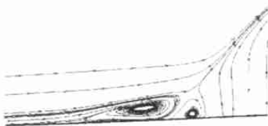
图 7 对称物面喷口上游流线图 Fig. 7 Stream lines before jet in symmetrical plane
