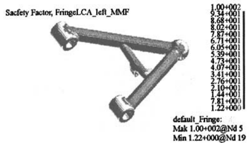
图9 10万km寿命安全系数分布 Fig.9 Distribution of safety factors under 100,000km fatigue life estimation
