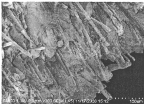
图 6 纤维增强 SiO 2 气凝胶复合材料断口形貌 Fig. 6 The fracture surface of fiber reinforced silica aerogel composites
