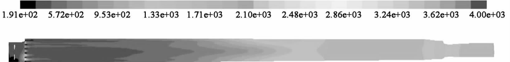
图 5 燃烧室内壁面温度分布 Fig.5 Contour of temperature on the inner surface of combustor
