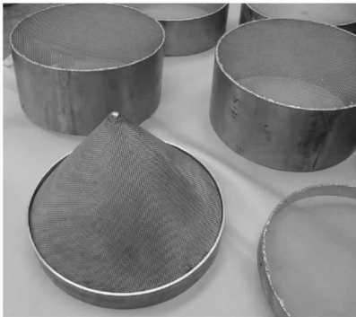
图 3 稳定段内上游组件 Fig.3 Upstream settling chamber components
