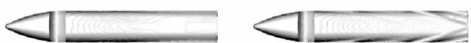
图 18 单子弹/组合子弹下表面压力云图 Fig. 18 Plot of under surface pressure cloud for the single bomb/the combined bomb
