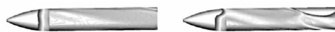
图 17 单子弹/组合子弹侧表面压力云图 Fig. 17 Plot of lateral surface pressure cloud for the single bomb/the combined bomb
