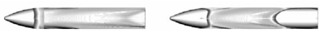
图 16 单子弹/组合子弹上表面压力云图 Fig. 16 Plot of upper surface pressure cloud for the single bomb/the combined bomb
