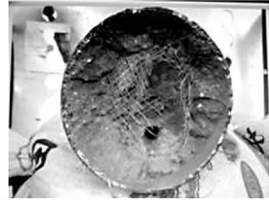
(b) 正面,次发 848.5m/s (b) Front face, second bullet at 845.5m/s
