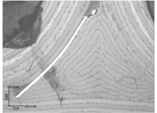
图1 含界面脱黏T型接头的微观形貌 Fig.1 Micro-structural features of composite T-joint with interfacial debonding
