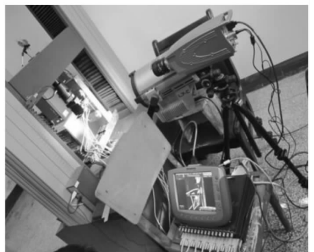
(b) 损伤实时监测装置 (b) Damage monitoring apparatus
