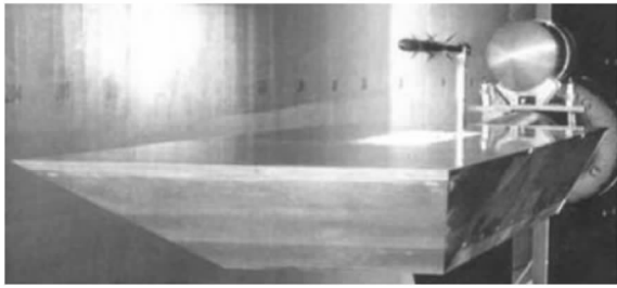
图1 M219空腔在DERA风洞噪声试验 Fig.1 Noise test of M219 cavity in wind tunnel
