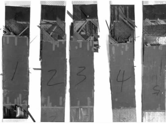
图7 阶梯挖补修复后试样拉伸破坏照片 Fig. 7 Photographs of tensile fracture of step-lap repaired specimens
