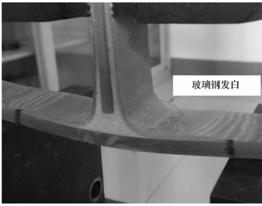
(a) 初始破坏 (a) Initial failure
