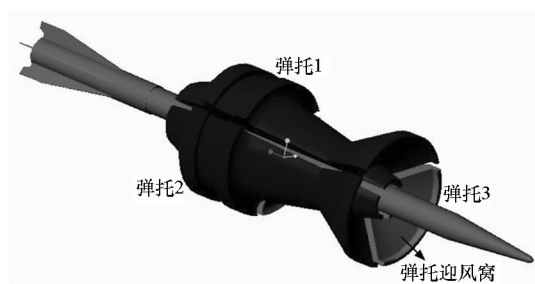
图1 尾翼稳定脱壳穿甲弹三维模型 Fig.1 Three-dimensional model of APFSDS
