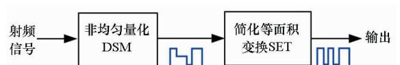
图 6 基于非均匀量化的脉冲编码策略 Fig. 6 Pulse encoding strategy based on non-uniform quantizing
