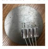
图 2 靶板背面热电偶测温点 Fig. 2 Thermocouple temperature measurement point on the back of the target
