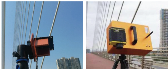
(a) MMW 雷达照片 (a) Picture of the MMW radar (b) K 波段雷达照片 (b) Picture of the K band radar
