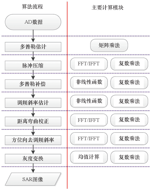
图 3 大斜视 SAR 成像算法流程及其主要计算模块 Fig. 3 Algorithm flow of high-squint SAR imaging and its main computing module
