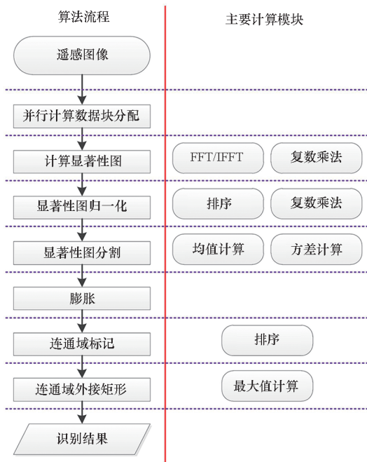
图 4 遥感光学图像目标识别算法流程及其主要计算模块 Fig. 4 Remote sensing optical image target recognition algorithm flow and its main computing module
