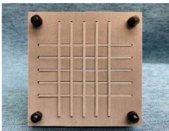
(b) 嵌入介质基板中的条形频率选择表面 (b) Bar shape frequency selective surface embedded in a dielectric substrate
