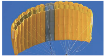
(c) 矩形翼伞 (c) Rectangular parafoil
