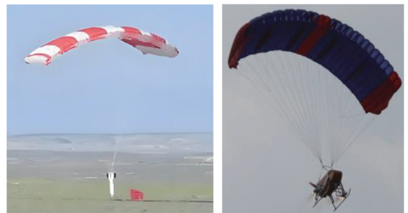
(c) 助推器翼伞回收 [15] (c) Parafoil recovery booster [15]
