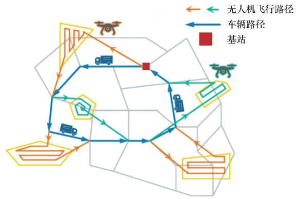
图 1 车辆支持的多无人机多区域覆盖路径规划问题 Fig. 1 Illustration of collaborative coverage path planning problem for multi-area by truck-supported multi-UAV
