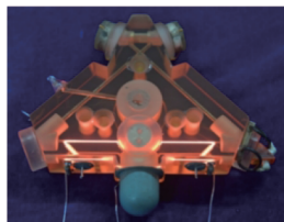
图 30 “全内腔”四频差动激光陀螺工程样机 Fig. 30 Engineering prototype of "full internal-cavity" four-frequency differential RLG
