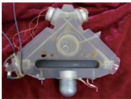
图 29 “准内腔”四频差动激光陀螺样机 Fig. 29 Prototype of "quasi-internal-cavity" four-frequency differential RLG
