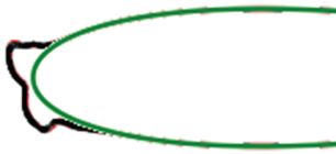
(a) \alpha = 2^\circ , v = 85 \text{ m/s} , T = -10 \text{ }^\circ\text{C} , MVD = 35 \text{ }\mu\text{m} , LWC = 0.7 \text{ g/m}^3 , t = 12.5 \text{ min}
