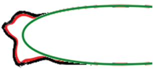
(c) \alpha = 2^\circ , v = 145 \text{ m/s} , T = -18 \text{ }^\circ\text{C} , MVD = 52 \text{ }\mu\text{m} , LWC = 0.6 \text{ g/m}^3 , t = 10 \text{ min}
