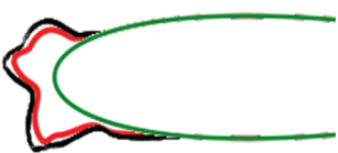
(d) \alpha = 2^\circ , v = 145 \text{ m/s} , T = -18 \text{ }^\circ\text{C} , MVD = 23 \text{ }\mu\text{m} , LWC = 0.7 \text{ g/m}^3 , t = 12.5 \text{ min}
