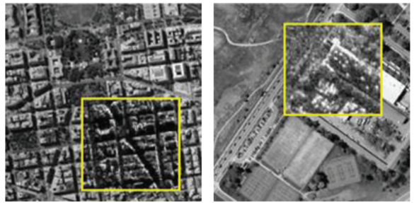
(a) SAR - 可见光(将 SAR 图像叠加到可见光图上) (a) SAR-visible (bottom layer is visible image; top layer is SAR image)
