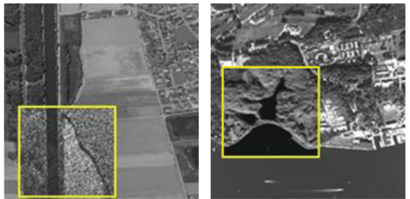
(b) SAR - 红外(将 SAR 图像叠加到红外图像上) (b) SAR-infrared (bottom layer is infrared image; top layer is SAR image)
