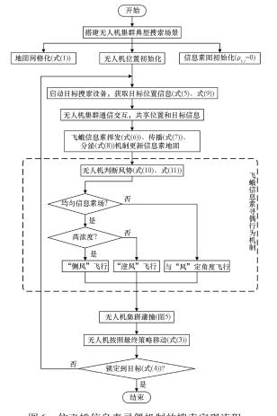
图 6 仿飞蛾信息素寻偶机制的搜索实现流程 Fig. 6 Search process based on moth pheromone courtship
